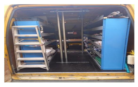
Improved vehicle racking will reduce stock damage, enable more effective van stock control, and reduce risks associated with manual handling injuries when removing materials and equipment from vehicles.
